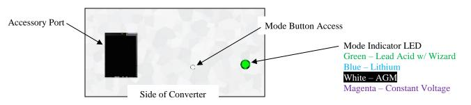
Press and hold the MODE BUTTON for at least 3 seconds until the LED changed color. Continue to depress button until the desire battery type is selected.
