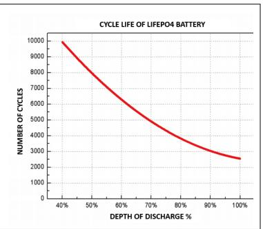
As the depth of discharge decreases, the cycle life gradually increases; 1C 100% DOD charge and discharge cycle life  $\geq$  2500 cycles; 1C 50% DOD charge and discharge cycle life  $\geq$  6000 cycles.
