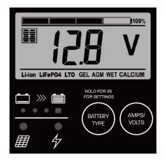
Press **BATTERY TYPE button** and hold for 3 seconds to go into your battery type selection mode, the battery type you select will be shown on the LCD meter, the default setting is AGM Battery; the controller will automatically memorize your battery type setting.
