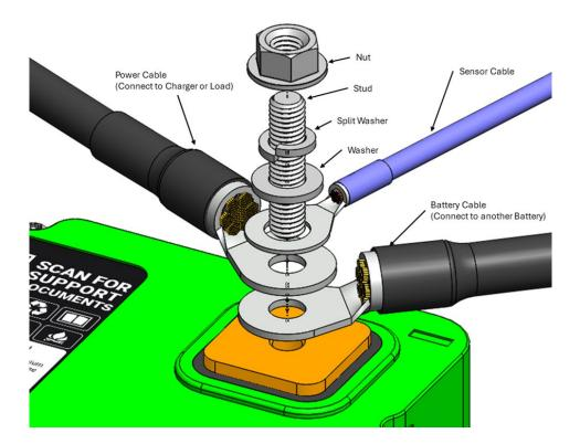
Torque to 8 lb-ft (96 lb-in). Do not finger-tighten. Do not over tighten. Check thread depth vs. bolt length. The female thread depth of the battery terminals is 12 mm.
