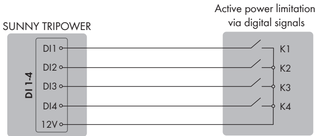
Figure 9: Connection of a signal source for active power limitation via digital signals (example)
