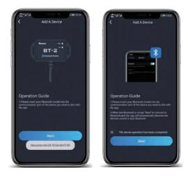
4.When a device is found, select the Bluetooth device, then name the device if you wish.Afterwards, press "Next" and then select the type of device you areconnecting. In this example, we will select Charge Controller.When successful, the App will confirm the product SKU. If the SKU is correct, click"OK" to start communicating with your Rover 30Amp.
