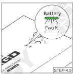
After waiting for 15S, the Battery indicator flashes green and the battery charger starts to work.
