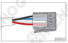
Insert the bare wires of the Drop Cable (sold separately) all the way into the wire ports of the Drop Plug (not included) following the Drop Plug pinout. The red PS+ wire goes to pin 1, the white CAN\_H wire goes to pin 2, the blue CAN\_L wire goes to pin 3, and the black PS-wire goes to pin 4.
