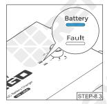
When the power of the starting battery is low, the battery charger will automatically reverse charge the starting battery from the service battery system, and the Battery indicator lights up blue and remains solid.
