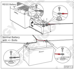
Connect the voltage sensor ring terminal to the positive/ negative pole of the battery system.
