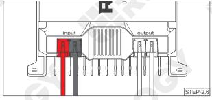
Insert the Anderson PP75 connectors into the Input terminal.
