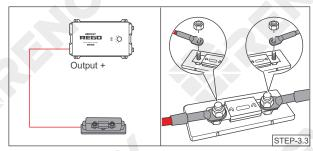
For your safety, it is recommended to use a battery fuse (80A). Connect the positive Battery Adapter Cable (output) to one end of the battery fuse, and then connect the other end to the positive bolt of the battery.
