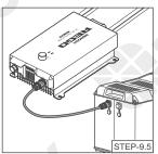
Connect REGO devices in series through either of the CAN Communication Ports with the Communication Cables (sold separately).
