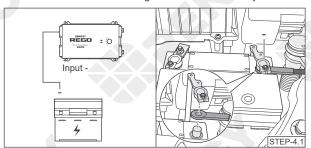
Attach the ring terminal of the negative Battery Adapter Cable (input) to the negative bolt of the starting battery.
