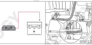
Attach the ring terminal of the positive Battery Adapter Cable (input) to the positive bolt of the starting battery and tighten with a wrench.
