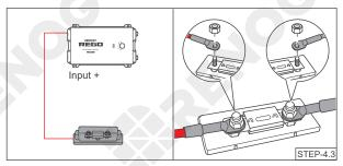
For your safety, it is recommended to use a battery fuse (80A). Connect the positive Battery Adapter Cable (input) to one end of the battery fuse, and then connect the other end to the positive bolt of the starting battery.
