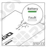
Once the battery wiring is completed correctly and the battery is turned on, the battery charger's Battery indicator lights up green.
