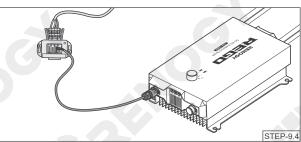
Connect either of the CAN Communication Ports of the battery charger to the drop socket on the drop tap with the Drop Cable.
