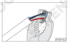
Squeeze the crimp area of the Drop Plug with a pair of split joint pliers.
