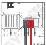
Insert the Anderson PP75 connectors into the Output terminal.
