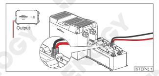
Insert the Anderson 120 connector of the Battery Adapter Cable (output) to the System Combiner Box.
