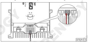
Insert the voltage sensor terminal block to the BVS port.
