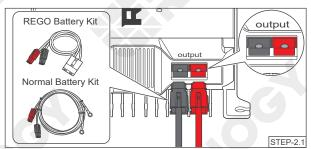
For the Output terminal, align the Battery Adapter Cable's Anderson PP75 connectors to the correct orientation and polarity.
