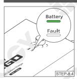
Under normal conditions, the Fault indicator will not light up.
