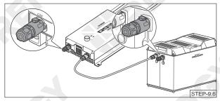
Plug the Termionator Plug (sold separately) into the free CAN Communication Ports on the first and last REGO devices.
