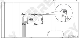
Place the battery charger against a flat surface and secure it with included screws.
