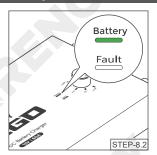
Once the service battery system is fully charged, the battery charger stops working and the Battery indicator lights up green and remains solid.
