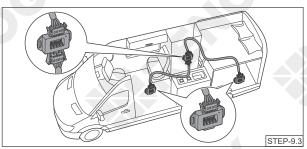
Locate the drop tap (not included) on the RV-C bus (not included) that is the closest to the battery charger installation location. The drop taps are usually located above the entry door, in the bathroom, or under the bed in the RV.
