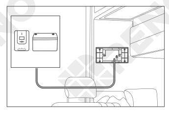
1. Ensure the selected communication cable is long enough to connect Renogy ONE to other devices.
