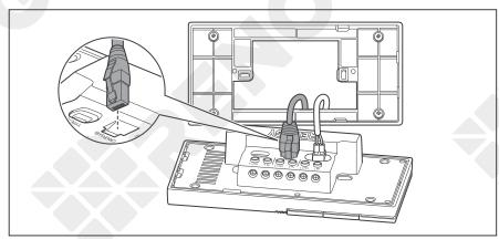
Connect the preembedded RJ45 connector to the RJ45 port of Renogy ONE.
