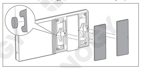
3. Align the snaps on the back of the panel switches, and press the switches until they "click".
