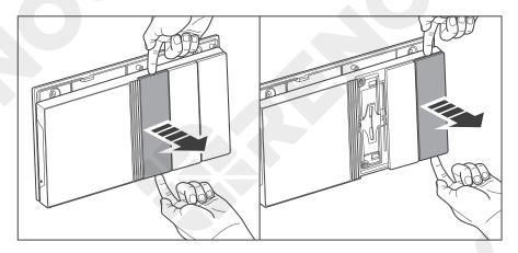
Disassemble Panel Switch
