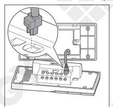
2. Insert the 12V power cable terminal block into Power Port of Renogy ONE.
