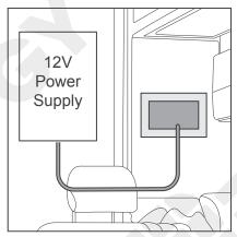
2. Tape the mounting template to the selected mounting location, and measure whether the 12V power cable is long enough to connect Renogy ONE to your DC power supply. If the included 12V power cable is not long enough for connecting Renogy ONE to your DC power supply, re-select a mounting position or use an extension cable (≥ 22 AWG). If you do not need to extend the 12V power cable, go to <a href="Step 5">Step 5</a>.
