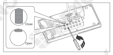
Use a Phillips screwdriver to turn the wire hatch screw counterclockwise.
