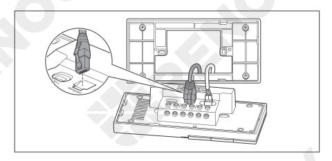
Connect the preembedded RJ45 connector to the RJ45 port of Renogy ONE.
