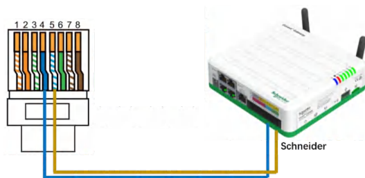
Connect with Schneider inverter/charger
