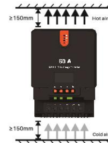
Fig. 2.1 Installation and heat dissipation
