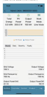
As shown in the figure below, in the red box area, you can view the total power generation data, input and output power data of the current equipment, and the working mode of the equipment.
