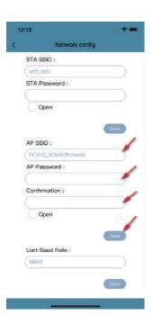
Step 8: After entering the value of the baud rate, click the "Save" button to complete the setting of Uart Baud Rate.
