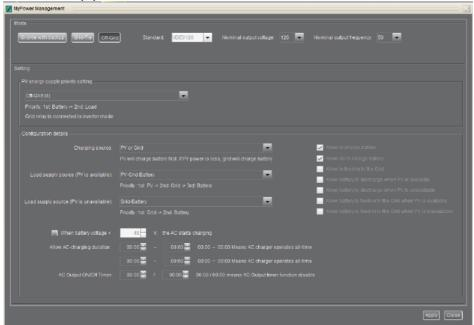
PV energy supply priority setting: 1st Battery, 2nd Load
