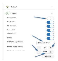
Click the Output tab pointed out by the red arrow, and after the blue arrow sets the parameters under Output, click the Apply button to complete the setting of the parameters of the Output tab.
