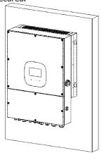
2. Raise the inverter and place it over the four screws.
