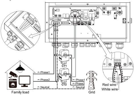
**Step 2:** Power on the inverter, wake up the LCD and modify LCD setting. Enter LCD program #13 and set up as any Grid-tie with backup mode. The CT will not be enable if not setting to grid-tie with backup.
