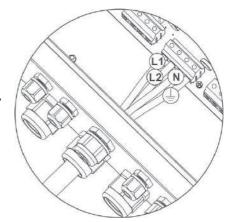
**CAUTION:** Do NOT connect the utility to "AC Output Connector (Load connector)". **CAUTION:** Be sure to connect L terminal of load to L terminal of "AC Output Connector(Load connector)" and N terminal of load to N terminal of "AC Output Connector(Load connector)". The G terminal of "AC Output Connector" is connected to grounding of the load. Do NOT mis-connect.
