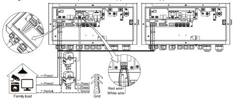
**Step 2:** Power on all inverters, wake up the LCD and modify the Settings. Enter LCD program #13 and set up as any Grid-tie with backup mode. The CT will not be enabled if not setting to grid-tie with backup.
