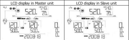
Step 5: If there is no more fault alarm, the parallel system is completely installed. Step 6: Please switch on all breakers of Line wires in load side. This system will start to provide power to the load.
