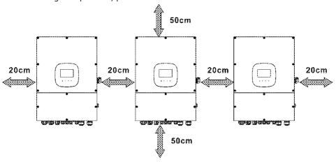
**NOTE:** For proper air circulation to dissipate heat, it's necessary to allow a clearance of approx. 20 cm to the side and approx. 50 cm above and below the unit. Be sure to install each unit in the same level.
