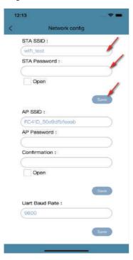
Step 7: Enter the Wi-Fi name (AP SSID) and Wi-Fi password (AP Password) of the Wi-Fi card, confirm the password again and click the "Save" button to complete the setting of the Wi-Fi card.
