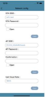
Step 6: Enter your Wi-Fi name (AP SSID) and Wi-Fi password (AP Password), then click the "Save" button to complete the setting.
