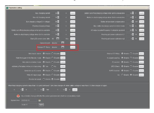
After CT function is enabled, program# 14 will be automatically changed to HBD2, program #15 will automatically set to turn off AC charging and program #16 will be disabled feed-in function.
