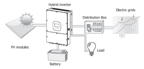
Figure 1 Basic hybrid PV System Overview
