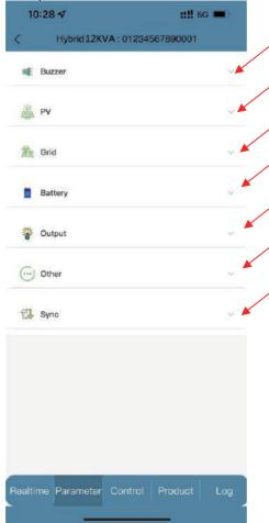
Click the Buzzer tab indicated by the red arrow, and after the blue arrow sets the parameters under Buzzer, click the Apply button to complete the setting of the Buzzer tab parameters.
