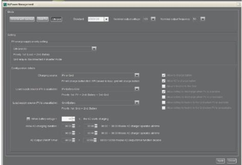
PV energy supply priority setting: 1<sup>st</sup> Load, 2<sup>nd</sup> Battery
