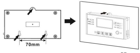
Note: Wall installation should be implemented with the proper screws to the right.
