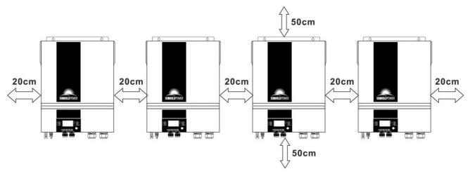
**NOTE:** For proper air circulation to dissipate heat, allow a clearance of approx. 20 cm to the side and approx. 50 cm above and below the unit. Be sure to install each unit in the same level.
