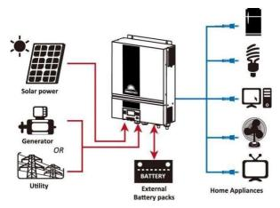
Figure 1 Basic hybrid PV System Overview
