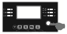
Step 5. Be sure to select battery type as "PYL" in LCD program 5.
