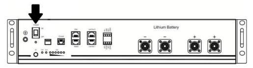
Step 3. Press more than three seconds to start Lithium battery, power output ready.
